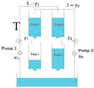
Quadruple Cylindrical Tank Process
